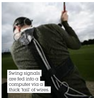
A small transmitter generates an electromagnetic field in which you stand and swing.
